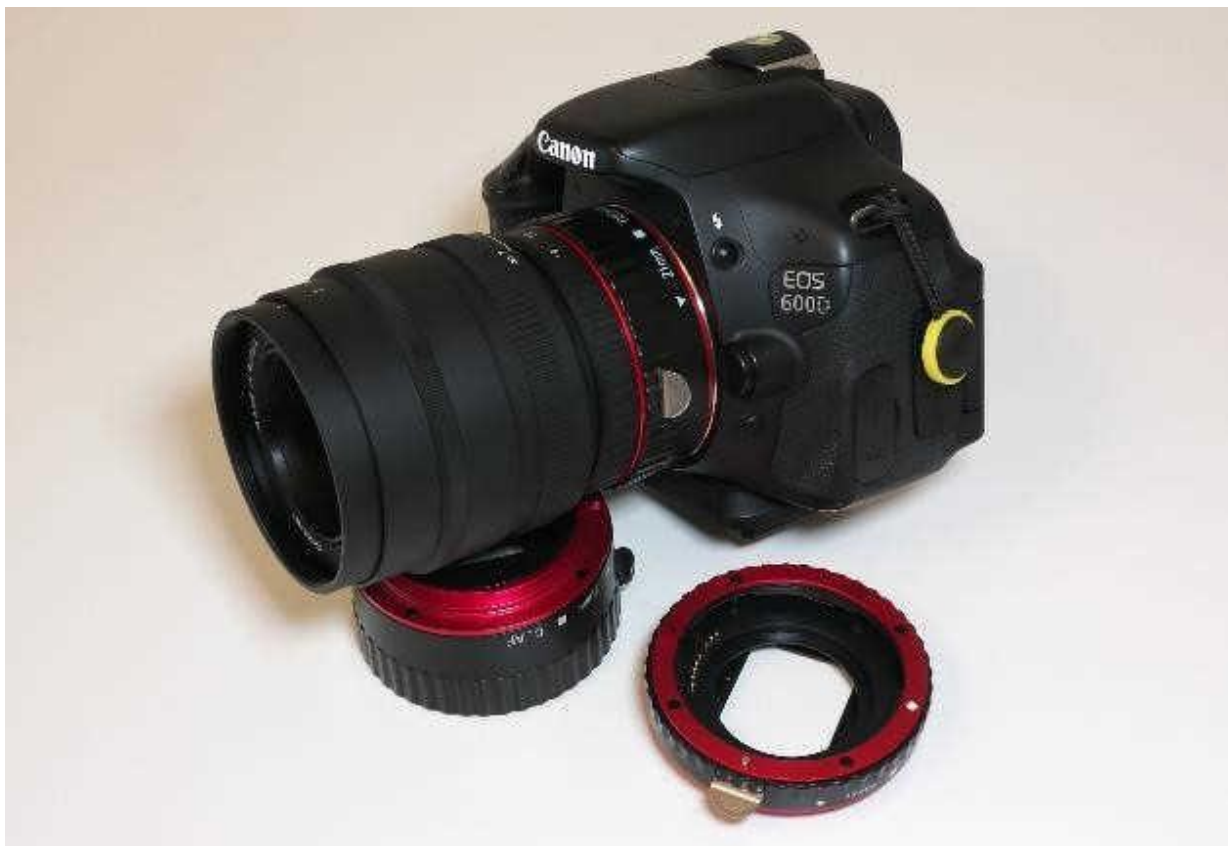
Figure 15. Mounting the Selenia 58mm f/1.9 lens to the camera with extension tubes.
