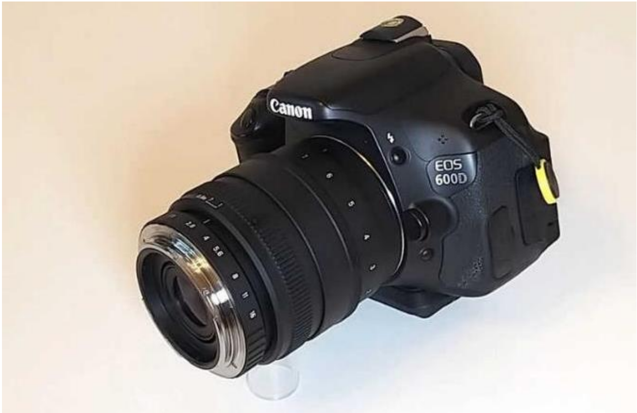
Figure 18. Attaching the Selena 58mm f/1.9 lens to the camera with the reverse macro adapter. Quite a large magnification can be obtained with this method (fig. 19).
