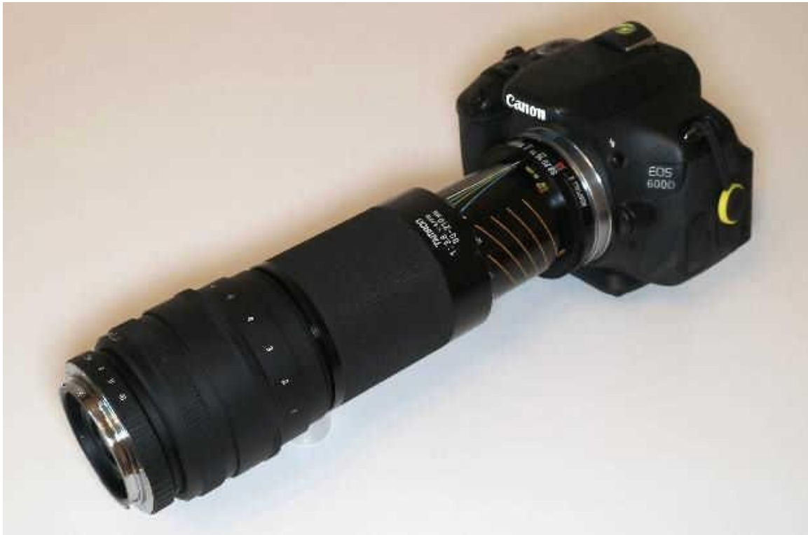
Figure 21. Using reversing (coupling) rings to connect Selenia 58mm f/1.9 and Tamron-103A 80-210mm f/3.8-4 lenses.
