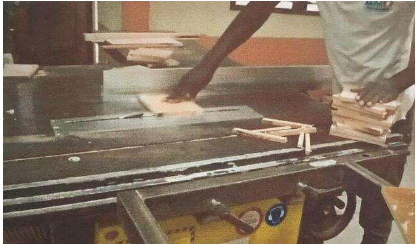
Figure 27. Cutting and template grooving of addition machine.
