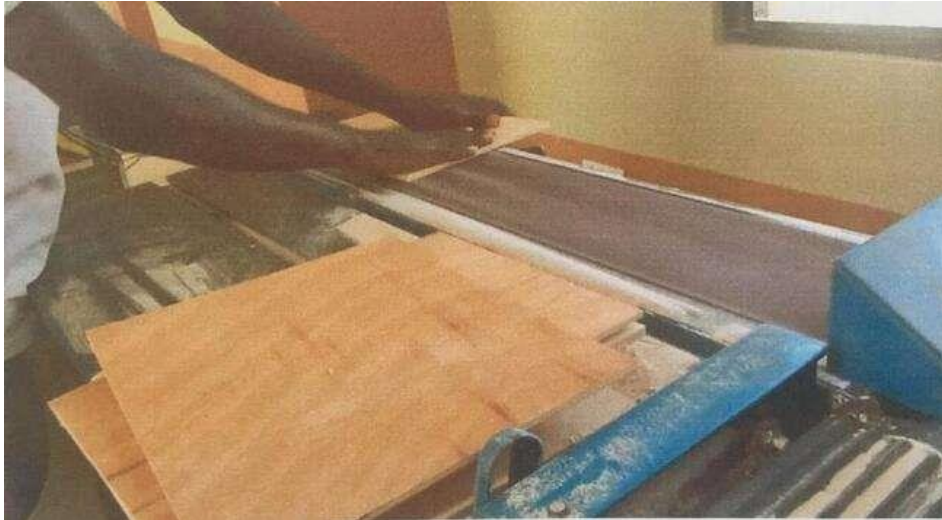
Figure 11. Cutting and sanding of wooden boards on the sander.
