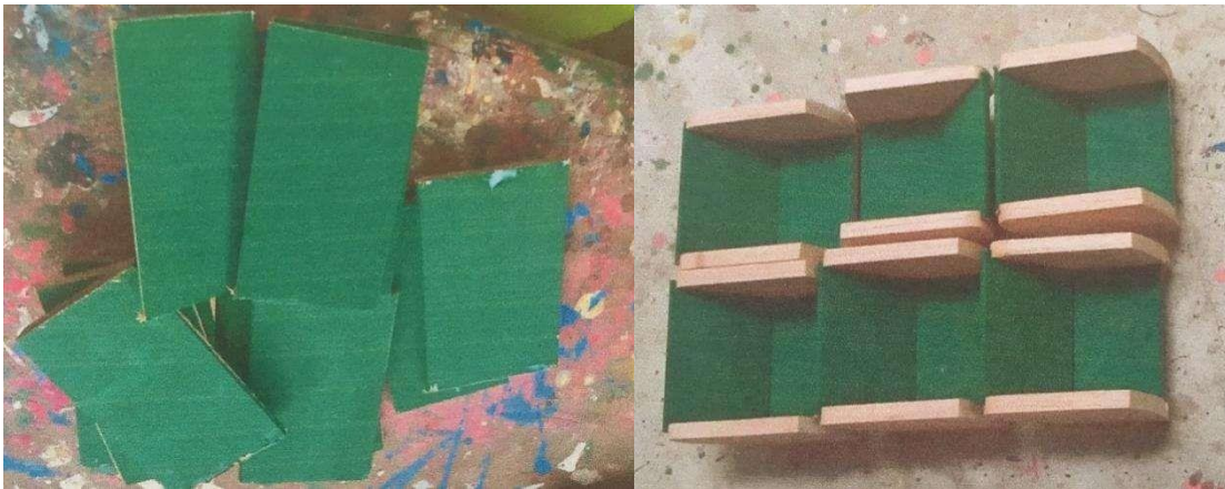
Figure 28. Cut and joint parts to form the final collector.
