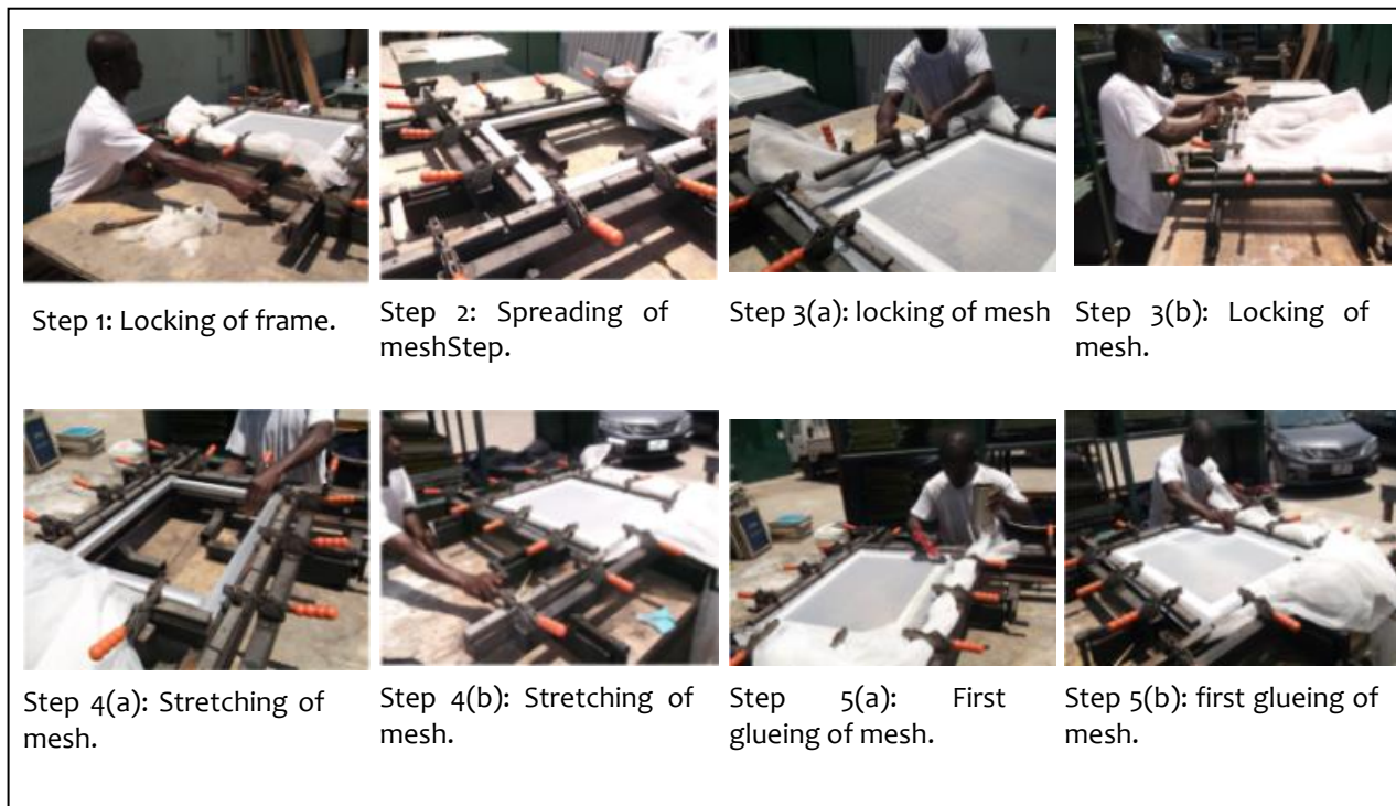
Figure 4.3. Processes of Stretching Aluminum Frame.
