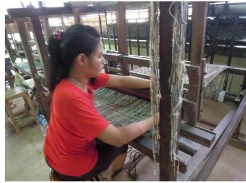
Figure 5. Process of Weaving Yarns into Fabric Using Non-machine Weaving Equipment (ATBM) at the Tarum Bali
