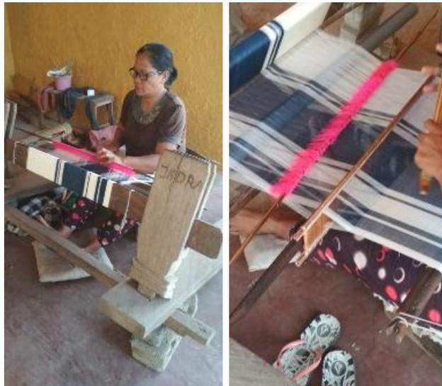
Figure 6. Process of Weaving Yarns into Fabric Using Gedhog Weaving Equipment at the Surya Indigo Workshop
