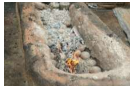
Figure 1.36: Moulds in “dewaxing” furnace.
