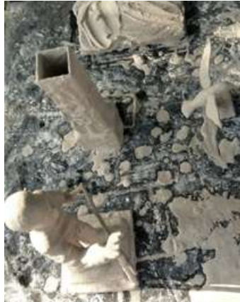
Figure 1.28c: Coating of wax models
