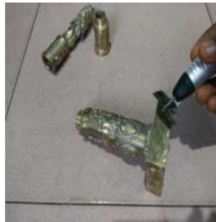
Figure 1.47b: Polishing with a flex shaft.
