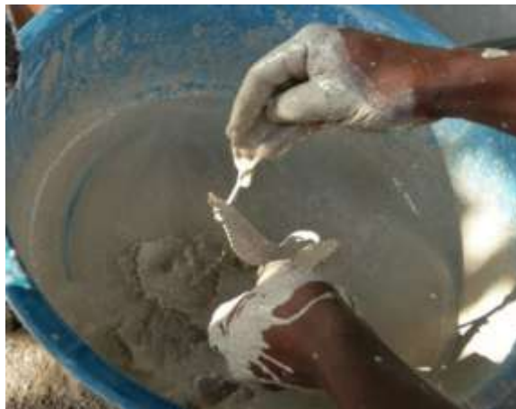
Figure 1.28c: Coating of wax models
