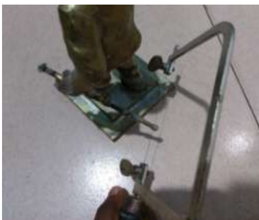
Figure 1.40: Cutting excess metal with a jeweler’s saw
