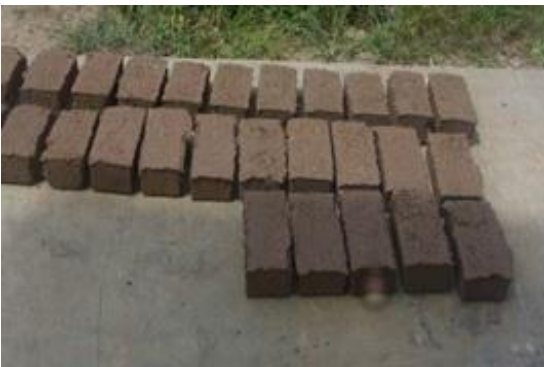
Plate 25: Wet manufactured bricks on platform to dry.
