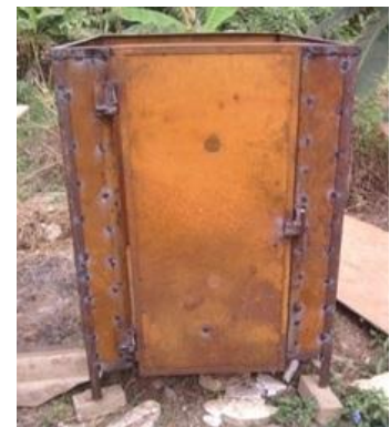
Plate 31: Welded galvanized sheet to the frame.
