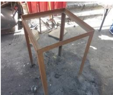
Plate 29: Skeletal structure of the kiln
