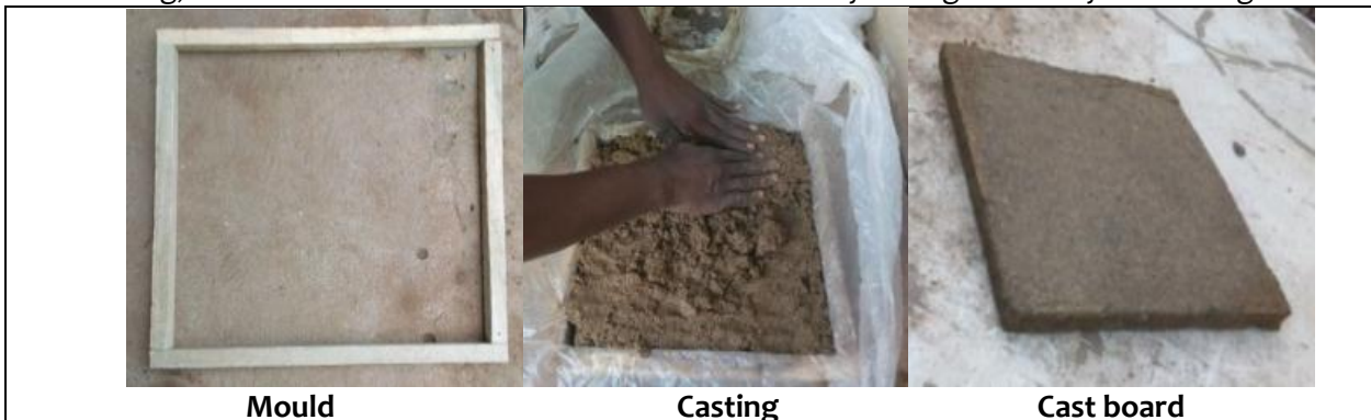
Figure 10: Casting a board in bond groundnut shell powder
