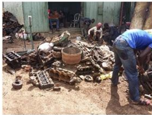
Figure 3: Breaking down cast iron scraps
