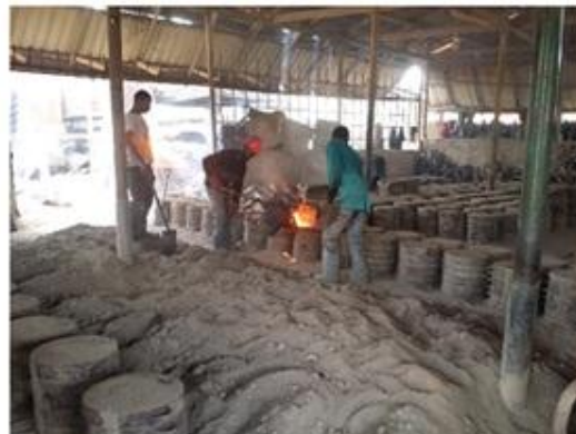
Figure 5: Feeding moulds with molten metal
