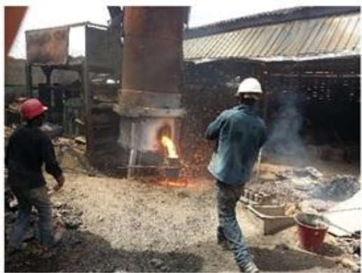
Figure 4: Collecting molten metal
